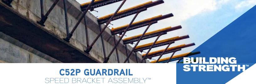
The C-52P Guardrail Speed Bracket Assembly is designed for fast and easy attachment to the C-49 Bridge Overhang Bracket. The C-52P's Speed Bracket bolts securely to the C-49 Bridge Overhang Bracket and provides a base to simply install the Guardrail Post. The Guardrail Post has a nail down feature to prevent uplift.
