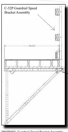
\*WARNING: Guardrail Speed Bracket Assembly must be secured to deck with proper fasteners to ensure complete safety.
