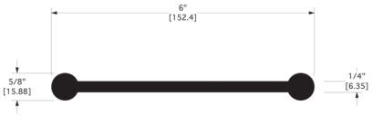
PVC647 6" Dumbbell Waterstop 100 ft Head of H 2 O • 50 lft/roll • .71 lbs/lft
