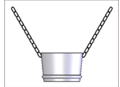
Steel Collar connects to the Tremie Pipe with chains.
