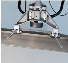
Durable stainless steel mounting levers allow for tool-less board removal.
