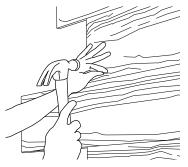
1) Fasten boards to formwork Set up one side of formwork (the side where the board form will be attached) and nail boards to wall.
