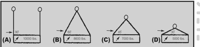
Example: Using the above reference, load lifted is 10,000 lbs.
