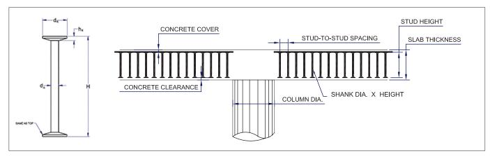
Anchor Size (H) + Concrete Cover + Concrete Clearance = Slab Thickness
