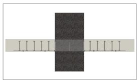
With Stud Rail in place, the shear stress is transferred to a larger area around the column.
