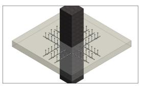
Without Stud Rail, the deck-to-column connections are prone to punching shear failure.
